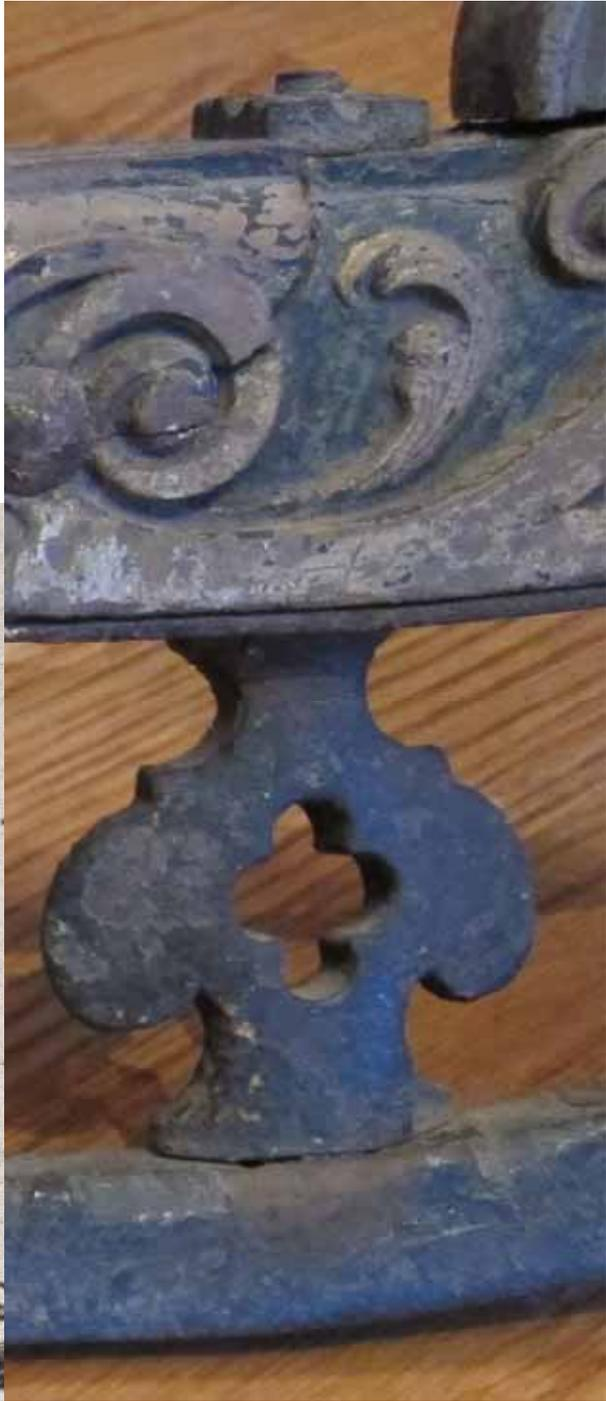
There are sprung devices (now shortened) beneath the driver's perch that punched into the snow or ice to aid turning or braking when the driver stood on them.
